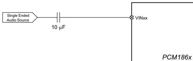
Figure 54. Analog Input Circuit for Single Ended Input Applications
